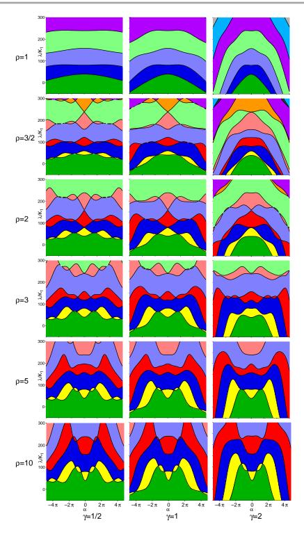
**Figure 6.1.** The index on the plane of unbuckled equilibria for various values of  $\rho$ , the ratio of bending stiffnesses, and of  $\gamma$ , the ratio of twisting to bending stiffness. In each graph, the index of the unbuckled equilibrium with twist angle  $\alpha$  and endloading  $\lambda$  is indicated by color, following the scheme in Figure 6.2. Black curves indicate the set of branch points as determined by the analysis in sections 6.1 and 6.2.
