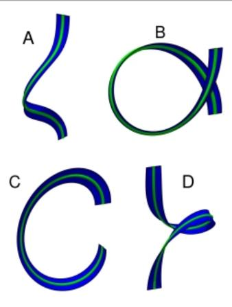
**Figure 7.3.** Physical configurations appearing in the bifurcation diagrams in Figure 7.2. The centerline of the strut is shown as a green tube, while the director  $\mathbf{d}_1$  is shown as a blue ribbon.
