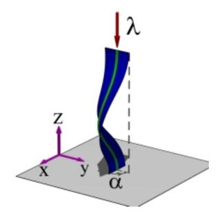
**Figure 1.1.** An elastic strut clamped at each end, with a relative twist angle  $\alpha$ , and with one end allowed to slide vertically in response to an imposed force  $\lambda$ . The cross-sections of the rod are elliptical, which we depict by showing the curve through the centers of the cross-sections as a green tube and tracking the major axes of the cross-sections with a blue ribbon.
