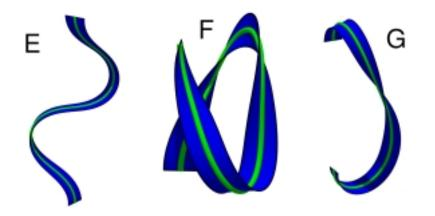
**Figure 7.5.** Physical configurations appearing in the bifurcation diagrams in Figure 7.4. The centerline of the strut is shown as a green tube, while the director  $\mathbf{d}_1$  is shown as a blue ribbon.
