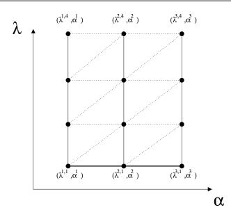
**Figure 7.6.** Triangulation of plane of unbuckled equilibria: The solid horizontal line at the bottom of the grid represents the initial calculation fixing  $\lambda$  and allowing  $\alpha$  to vary. Each of the solid vertical black lines represents a continuation in  $\lambda$  keeping  $\alpha$  fixed. Each  $(\lambda^{i,j}, \alpha^i)$  is marked with a black circle, and the triangulation is shown with the dotted lines.
