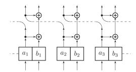
FIG. 7. One-dimensional radius-1/2 QLGA from permutation of bits in the CA of Figure 6.
