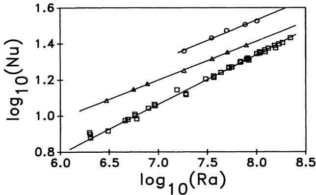
FIG. 10. Scaling of  $Nu$  with  $Ra$ , with nondimensional forcing  $v_f d/\kappa$  held constant at the following values: zero ( $\square$ ),  $9.4 \times 10^3$  ( $\triangle$ ), and  $3.0 \times 10^4$  ( $\circ$ ). The heat flux is increased (and the slope reduced) by the forcing (upper two curves).
