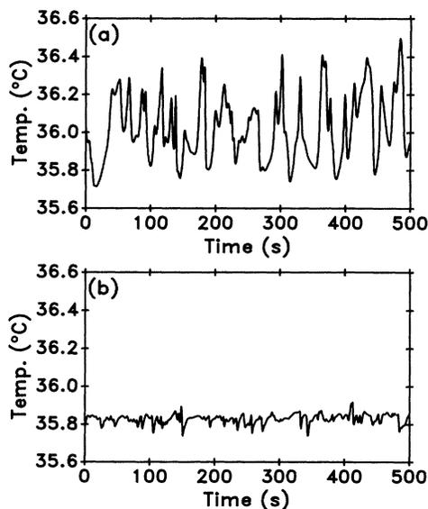
FIG. 7. Temperature time series measured at the lower probe, at  $Ra = 5.2 \times 10^7$ . (a) Unperturbed convection. (b) Time-independent forcing by a single vortex with  $v_f = 3.2$  cm/s. Warm temperature excursions are almost completely absent in (b), indicating a nonbursting lower boundary layer.
