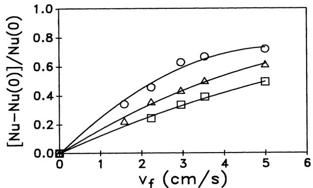
FIG. 9. Enhancement of the Nusselt number  $Nu$  by many-vortex forcing:  $Ra = 1.8 \times 10^7$  ( $\circ$ ),  $Ra = 5.0 \times 10^7$  ( $\triangle$ ),  $Ra = 1.0 \times 10^8$  ( $\square$ ). Curves are drawn through the data to guide the eye.
