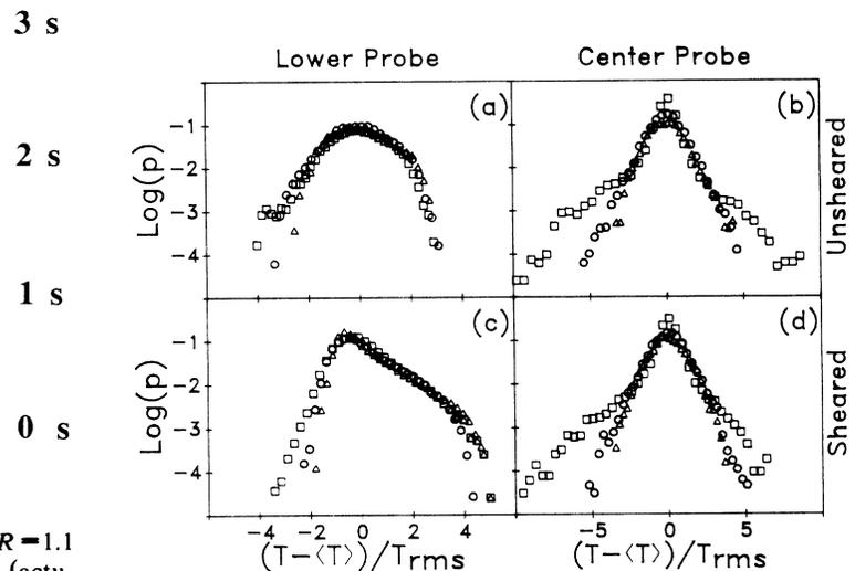
FIG. 5. Temperature probability distribution functions:  $R=4.9 \times 10^6$  ( $\square$ ),  $5.7 \times 10^7$  ( $\Delta$ ),  $1.1 \times 10^8$  ( $\circ$ ). The data are scaled by subtracting the mean temperature  $\langle T \rangle$  and dividing by the rms temperature fluctuations  $T_{rms}$ . (a) Unsheared, lower probe; (b) unsheared, center probe; (c) sheared (6 mm/s), lower probe; (d) sheared, center probe.
