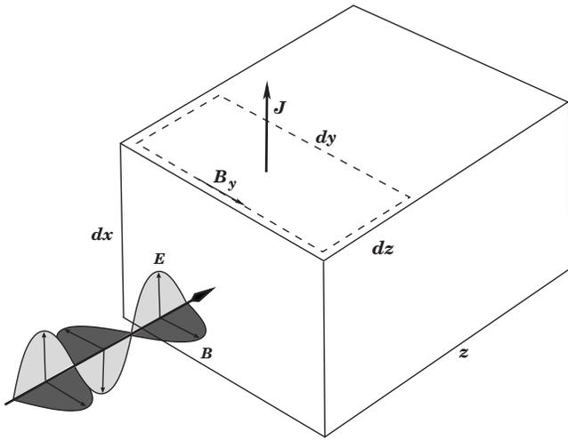
Fig. 5. A light wave traveling in the  $z$ -direction strikes an almost perfectly conducting mirror of thickness  $z$ , width  $dy$ , and height  $dx$ . An Ampèrian loop in the  $yz$  plane is also shown, with the direction of  $\mathbf{B}$  given by the right-hand rule.
