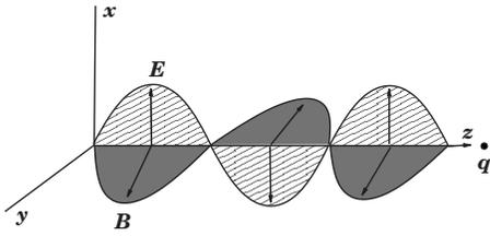
Fig. 1. An electromagnetic wave traveling in the  $z$ -direction strikes a point particle with charge  $q$ . The  $E$ -field is taken in the  $x$ -direction and the  $B$ -field is taken in the  $y$ -direction.
