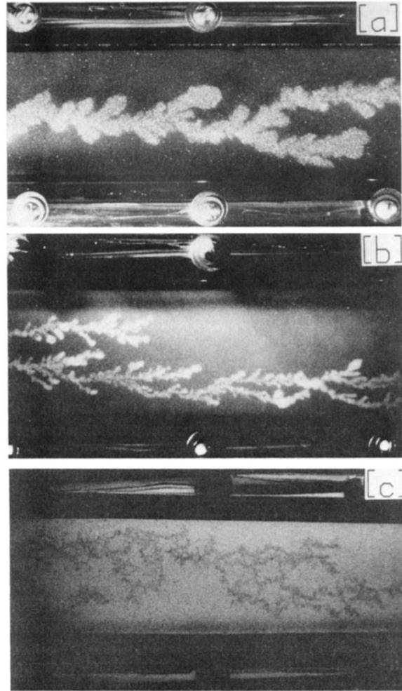
FIG. 1. (a) Wetting displacement with water (light color) displacing oil (dark). Here  $d=0.5$  mm ( $\kappa=2\times 10^{-6}$  cm<sup>2</sup>) and  $N_{Ca}=6.9\times 10^{-4}$ . (b) Wetting displacement with  $d=0.15$  mm ( $\kappa=2\times 10^{-7}$  cm<sup>2</sup>) and  $N_{Ca}=3.8\times 10^{-4}$ . (c) Nonwetting displacement with oil (dark) displacing water and glycerol (light). Here  $d=0.5$  mm ( $\kappa=2\times 10^{-6}$ ) and  $N_{Ca}=2.3\times 10^{-4}$ .  $M\approx 200$  in all cases.
