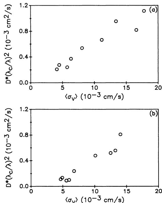
FIG. 5. Local transport enhancement as a function of the amplitude of local time dependence at  $R/R_c=26.1$ . The effective diffusion coefficient  $D^*$  has been scaled to the critical wavelength  $\lambda_c$  for convection near onset. Each figure contains data from a single run. (a) Methylene blue dye. (b) Latex sphere impurity.
