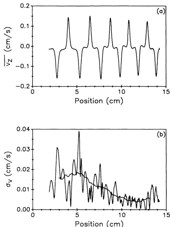
FIG. 1. LDV characterization of a time-periodic flow at  $R/R_c = 26.1$ . (a) Profile of the average vertical velocity  $\bar{v}_z(x)$ . (b) Standard deviation  $\sigma_v(x)$  of the local velocity. The smooth curve is the spatially averaged standard deviation  $\langle \sigma_v(x) \rangle$ .
