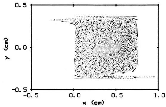
FIG. 7. Numerical determination of  $D^*$  by calculation of particle locations after one complete period of oscillation:  $A=0.14$  cm/s,  $\omega=0.49$  s $^{-1}$ ,  $2B/\lambda=0.02$ . Note the pinching of impurity near the roll corners (similar to that observed in Fig. 3).
