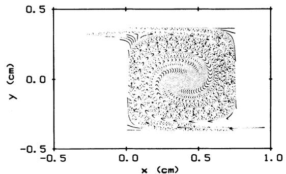
FIG. 7. Numerical determination of  $D^*$  by calculation of particle locations after one complete period of oscillation:  $A=0.14 \text{ cm/s}$ ,  $\omega=0.49 \text{ s}^{-1}$ ,  $2B/\lambda=0.02$ . Note the pinching of impurity near the roll corners (similar to that observed in Fig. 3).
