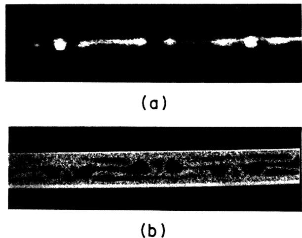
FIG. 9. (a) Shadowgraph image and (b) absolute value subtraction of two images separated time by one-half the period of oscillation at  $R/R_c = 32$ . (The convection cell is observed from the side and appears shallower than it actually is.) The motions of hot and cold fluid elements (dark spots in the image) can be seen clearly (b).
