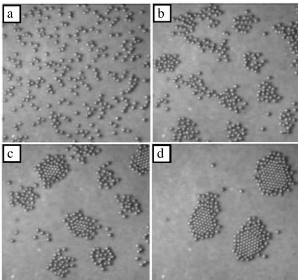
FIG. 2. Time evolution of an initially random distribution of beads. The attraction created by the streaming flow quickly collects the particles into clusters. ( $f = 50$  Hz,  $\Gamma = 4.5$ ) (a)  $t = 0$  s; (b)  $t = 8$  s; (c)  $t = 16$  s; (d)  $t = 32$  s.
