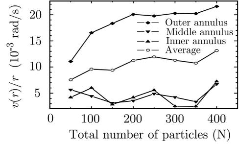
FIG. 4. Measured center-of-mass angular velocity  $v(r)/r$  [for  $f = 60$  Hz and  $A = 2g/(2\pi f)^2$ ] averaged (to reduce noise) over the three annuli described in the text for different numbers of particles. This angular velocity is greatest in the outer region.
