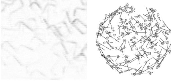
FIG. 3. (a) Still image of  $N = 200$  wires in the cell illuminated by visible light. (b) Vectors showing the total displacements of individual particles accumulated for 26.6 sec, with their initial positions marked as circles, for  $N = 350$ ,  $f = 60$  Hz, and rms vibrational amplitude  $A = 2g/(2\pi f)^2$ . In both (a) and (b), arm angle  $\alpha = -3\pi/4$ , stem length  $= 10.0 \pm 0.2$  mm, arm length  $= 4.0 \pm 0.2$  mm, and wire diameter  $= 0.91 \pm 0.05$  mm.
