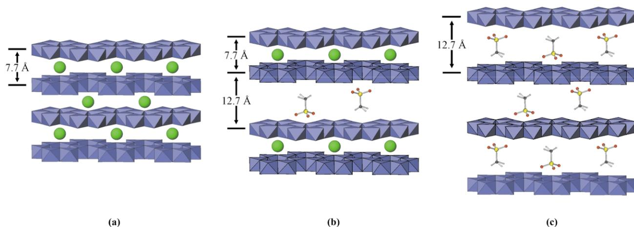
**Fig. 3** Schematic showing the intercalation of methylphosphonic acid: (a) The host lattice,  $[\text{LiAl}_2(\text{OH})_6]\text{Cl}\cdot\text{H}_2\text{O}$ ; (b) the second stage intermediate with alternate layers occupied by methylphosphonic acid and  $\text{Cl}^-$  anions; (c) the first stage product with all interlayer regions occupied by methylphosphonic acid.
