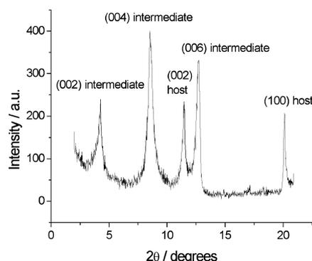
**Fig. 2** Powder XRD pattern of a quenched sample showing the presence of a second stage intermediate in the intercalation of MPA.
