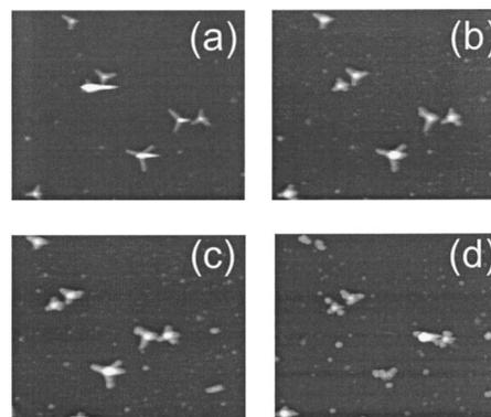
FIG. 3. Tapping mode AFM images ( $2.4 \times 2.1 \mu\text{m}^2$ ). (a) Initial image before application of forces. The tetrapod heights vary between 30 and 60 nm. (b) After a FV scan with maximum load of 50 nN. (c) After a FV scan at 90 nN. (d) Same after 130 nN. At this load the base arm structure is damaged.
