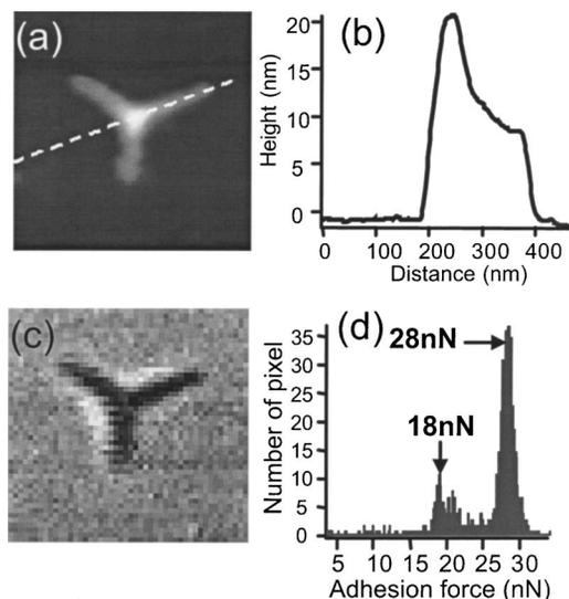
FIG. 2. (a) Topographic image of a tetrapod with a height of 25 nm, and height profile (b). (c) Adhesion force map extracted from the pull-off forces in a  $64 \times 64$  pixel force-volume experiment. (d) Histogram of adhesion forces showing a bimodal distribution.
