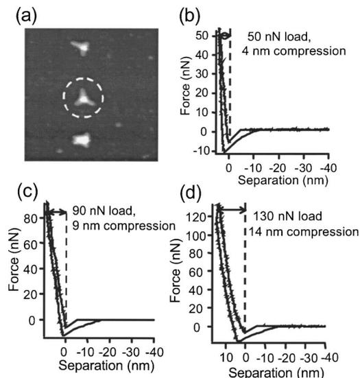
FIG. 4. (a) Tapping mode image ( $1.5 \times 1.5 \mu\text{m}^2$ ) containing three tetrapods with heights of 24, 25, and 25 nm. [(b)–(d)] Force-separation curves taken over the center of the tetrapod marked by the white circle in (a). The maximum loads are 50, 90, and 130 nN in each curve, respectively, which produced compressions of 4, 9, and 14 nm respectively.
