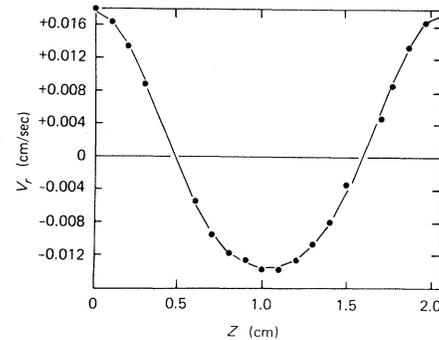
FIG. 2. Axial variation of the radial velocity for  $(f - f_c)/f_c = 0.014$ . The solid curve includes the fundamental term and a small second-harmonic term.
