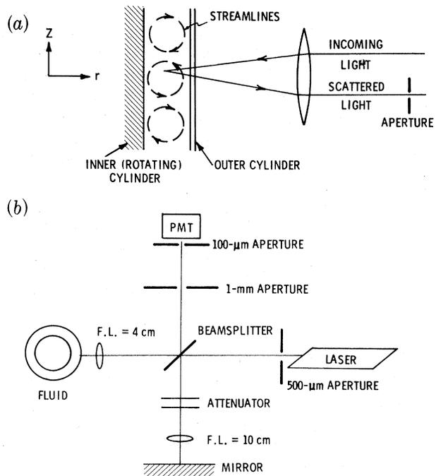
FIG. 1. (a) Side view of the cylindrical apparatus and light paths. The flow pattern shown schematically is actually superimposed on a much faster azimuthal flow perpendicular to the page. The axis of the rotating cylinder is along the  $z$  direction. (b) Top view showing the method used to mix the scattered and reference beams. Each arm is 30 cm long.
