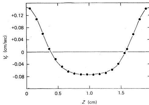
FIG. 3. Axial variation of the radial velocity for  $(f-f_c)/f_c=0.465$ . The solid line includes the fundamental and the second- and third-harmonic terms.
