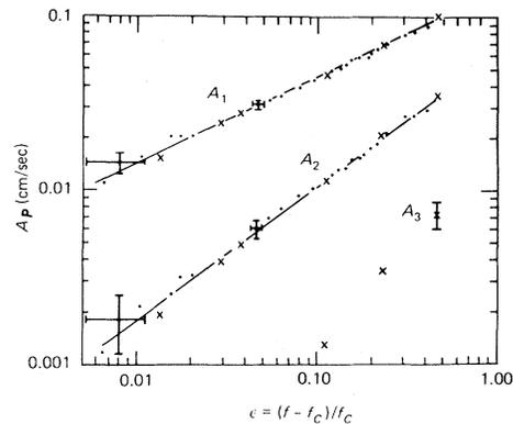
FIG. 4. Dependence of the Fourier coefficients  $A_p$  on the rotation rate. The solid lines represent the results of least-squares analyses, with  $f_c = 0.0651$  Hz.
