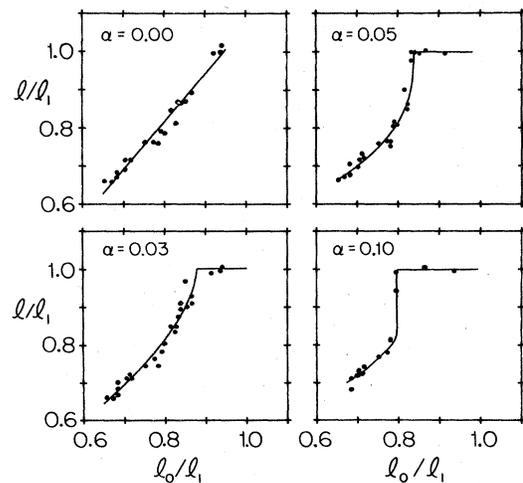
FIG. 6. Variation of the inverse  $l$  of the mean wave number with the unperturbed roll size  $l_0$  (in units of  $l_1$ ), for various forcing strengths  $\alpha$ . The  $C$ - $I$  transition is continuous for  $\alpha < 0.05$ , and discontinuous for  $\alpha > 0.05$ .
