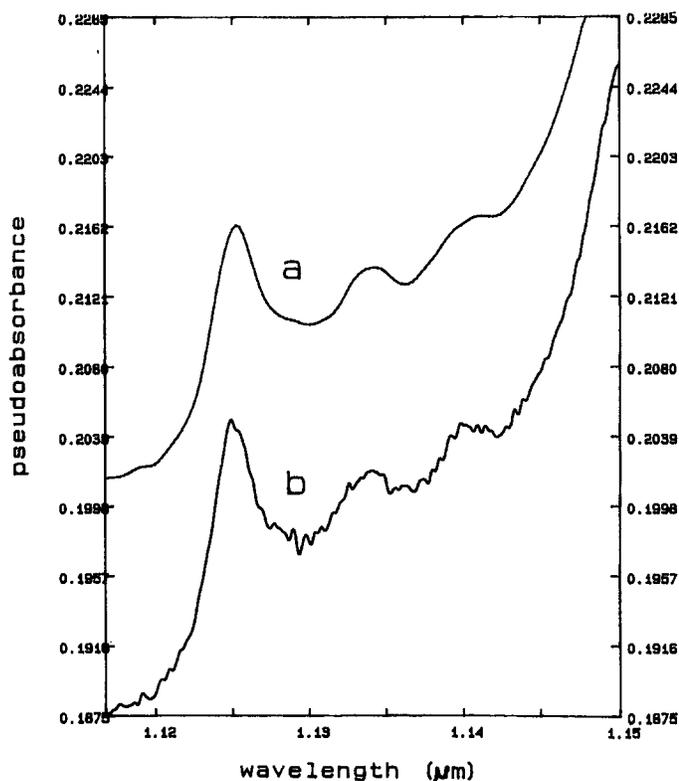
FIG. 12. A portion of the pseudoabsorbance spectra of crystalline glycine collected with different instrumental resolution: (a) 50-s scan at  $8\text{-cm}^{-1}$  resolution; (b) 6-min scan at  $2\text{-cm}^{-1}$  resolution. Spectral offset is arbitrary.
