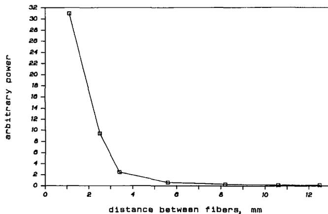
FIG. 7. Relative measured power from crystalline KCl obtained as a function of fiber separation within the dual-fiber probe where the probe rests on the surface of the specimen.
