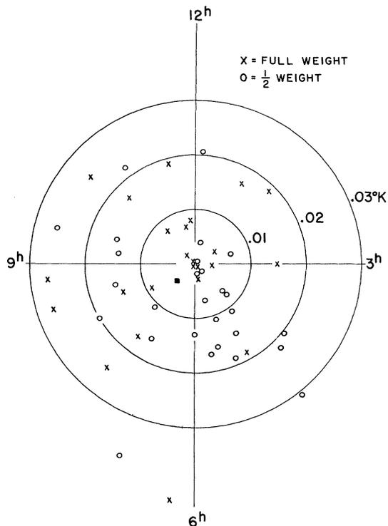
FIG. 2. The results of analyzing  $\sim 55$  isotropy runs for 12-h components. Half-weighted runs were interrupted by weather or instrument failure so that a complete 24-h series was not obtained. Note that the outer circle represents an amplitude of 1% of the background radiation temperature of  $3^{\circ}\text{K}$ . The average of all results is indicated by the solid square.
