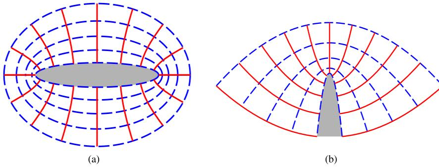
FIG. 10. Equipotentials (dashed blue) and field lines (solid red) for elliptical ((a), type  $*$ 2) and parabolic ((b), type  $*$ ) conductors. The equipotentials and field lines can be swapped for the elliptical conductors, giving rise to pairs of hyperbolic conductors.
