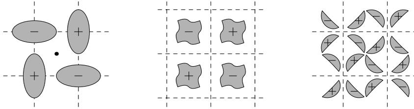
FIG. 8. Conductors having symmetry type  $4*2$  and color types  $2*22$  (left),  $442$  (center), and  $22\times$  (right). Individual conductors have symmetry types (tile groups)  $*2$  (left),  $4\bullet$  (center), and  $\bullet$  (right). Positively and negatively charged conductors are indicated by  $+$  and  $-$ , respectively.
