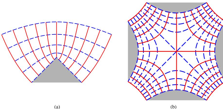
FIG. 11. Equipotentials (dashed blue) and field lines (solid red) for geometries described by Eq. (6). (a) An outside corner with  $n = 3/2$  and symmetry  $*$ . (b) A quadrupole lens with  $n = 1/2$  and symmetry  $*4$ .
