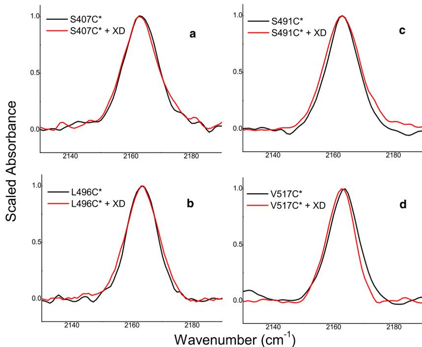
FIGURE 2 Infrared spectra in the C≡N stretching region for cyanylated N<sub>TAIL</sub> variants in the absence (black) and presence (red) of XD. (a) S407C\*, (b) L496C\*, (c) S491C\*, and (d) V517C\*.
