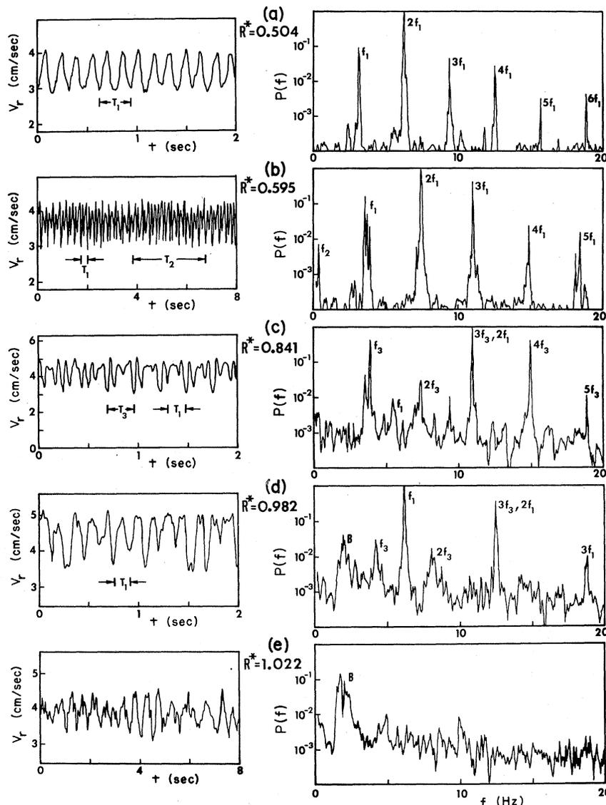
FIG. 1. Time dependence of the radial velocity and corresponding power spectra  $P(f)$  [with units  $\text{cm}^2 \text{sec}^{-2} \text{Hz}^{-1}$ , normalized so that  $\int_0^{25\text{Hz}} P(f) df = \langle (\Delta V_r)^2 \rangle$ ] for different reduced Reynolds numbers  $R^* = R/R_T$ .
