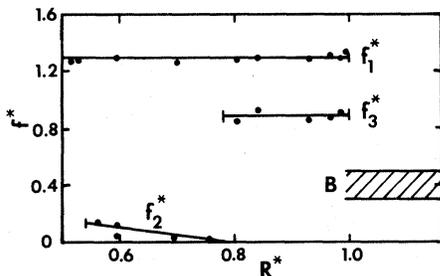
FIG. 2. The dimensionless frequencies  $f_i^* = f_i T$  as a function of  $R^*$ . The solid lines are to guide the eye, and the vertical bars demarcate the regions in which the  $f_i$  are present (except that the lower bound for  $f_1$  is  $R^* = 0.064$ ). The fact that  $f_1^* = 1.30$  and  $f_3^* = 0.87$  are constant indicates that  $f_1$  and  $f_3$  scale with rotation rate, whereas  $f_2$  does not.
