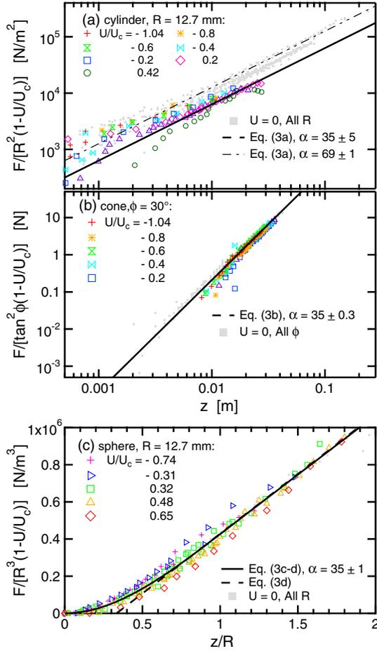
FIG. 2 (color online). Friction force versus depth for (a) cylindrical, (b) conical, and (c) spherical probes, normalized as in Fig. 1 and also by  $1 - U/U_c$ , where  $U$  is airspeed and  $U_c$  is airspeed at fluidization. The solid curves are simultaneous fits to Eq. (3) with  $\alpha = 35 \pm 5$ . All data from Fig. 1 are replotted as small grey points.
