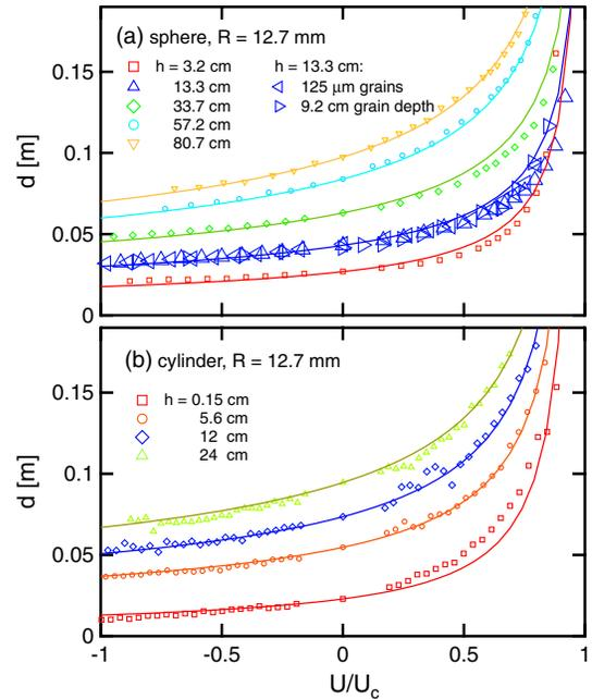
FIG. 3 (color online). Penetration depth versus normalized airspeed for (a) a sphere of mass 0.07 kg and (b) a cylinder of mass 0.2 kg, from various drop heights  $h$ . The grains are  $300 \mu\text{m}$  and the packings are 19.4 cm deep, except for two special cases in (a) where the depth and the grain size are decreased. The curves represent solutions of Eq. (2) and (a) in Eq. (3) with  $\alpha = 35$ , taking  $b$  to match the data at  $U = 0$ .
