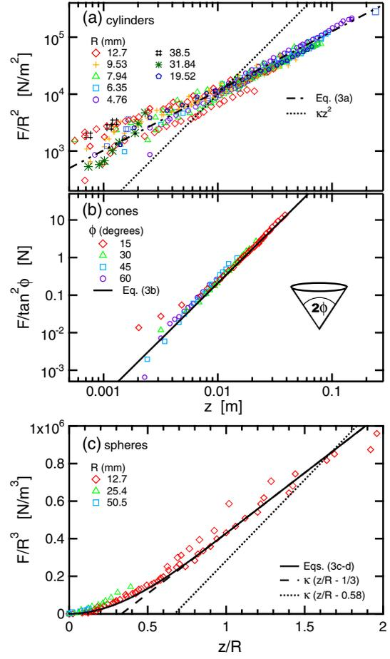
FIG. 1 (color online). Friction force versus depth for (a) cylindrical, (b) conical, and (c) spherical intruders of different geometry;  $R$  is radius and  $\phi$  is apex half-angle. The scaling of the y axes, and the curves through the data, are the expectations of Eq. (3) for  $d\mathbf{F}$  normal to the intruder surface area elements. The dashed (dotted) line in (c) represents expectation for  $z > R$  for  $d\mathbf{F}$  normal (tangential) to the intruder.
